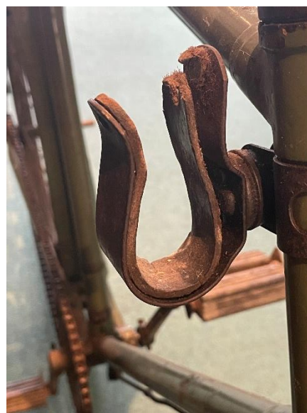
Close-up of rifle bracket on army bicycle
