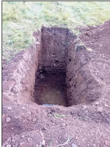
Trial Hole Inspection
