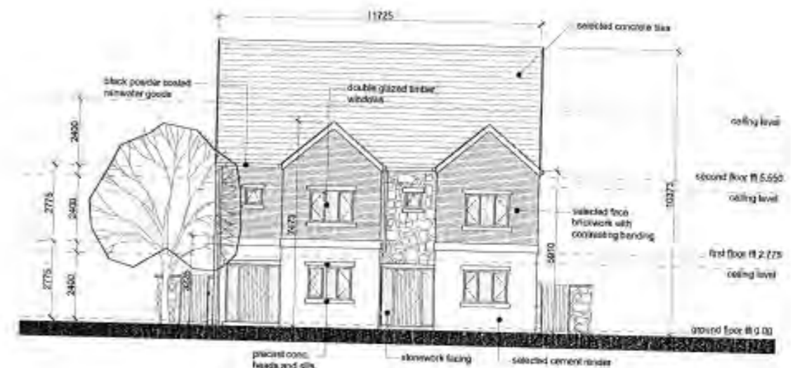
Previously Granted Typical Semi Detached House Type Elevation (Ref: 071311) by OBK Architects
