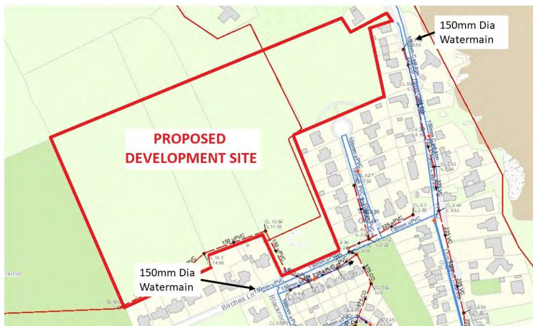
Figure 3 – Existing Water Supply
