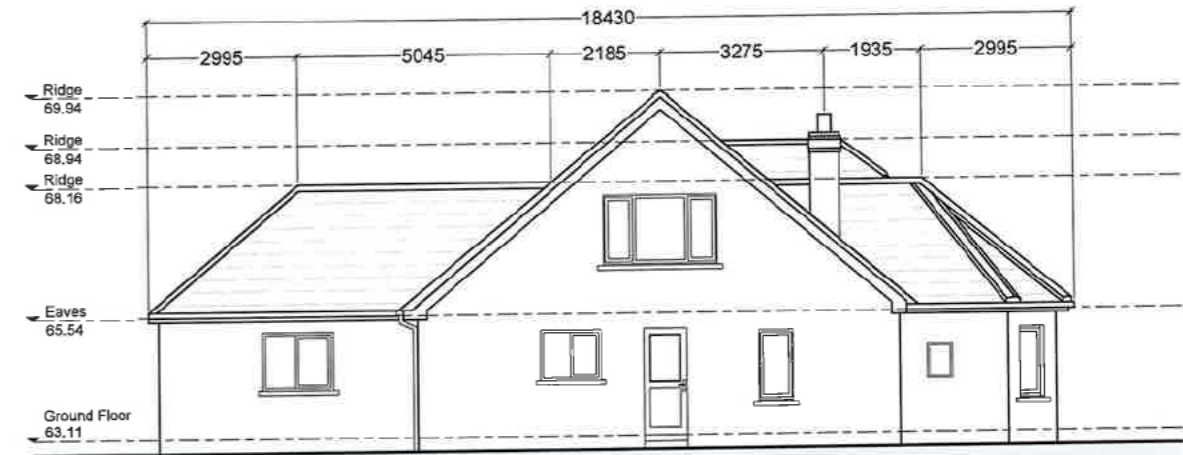
EXISTING MAIN HOUSE WEST ELEVATION SCALE 1:150@A3
