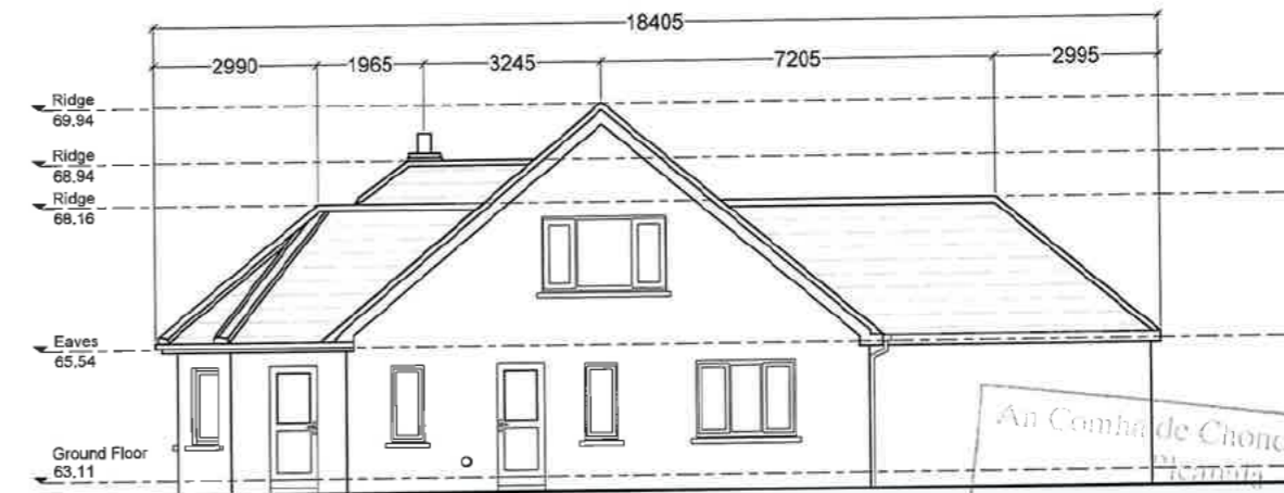
EXISTING MAIN HOUSE EAST ELEVATION SCALE 1:150@A3
